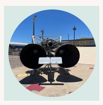
The Titan II missile used a **two-stage engine**. The **first stage engine** (left photo) burned for 2.5 minutes and consumed around 25,500 gallons (96,500 l) of fuel and oxidizer - around 170 gallons (640 l) per second. **Stage two** would ignite after stage one ran out of fuel. Then, explosive bolts would separate the two stages. Stage two (picture above) would burn for 3 minutes and bring the missile to an altitude of 200 miles (320 km). Stage 2 would turn off when on course.
