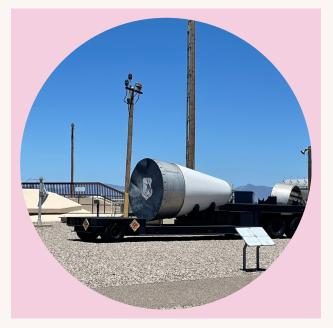
On the truck, you can see the **Re-Entry Vehicle (RV)**. It was built by General Electric, and it housed the **W-53 9 Megaton thermonuclear bomb**. The RV's name refers the fact that the RV would exit and reenter Earth's atmosphere, traveling at 16,000 mph (25,000 km/h). The RV did not have a guidance system, but it had thrusters that would adjust the trajectory. The RV's shell would also erode upon reentry, protecting the W-53 bomb from damage.
