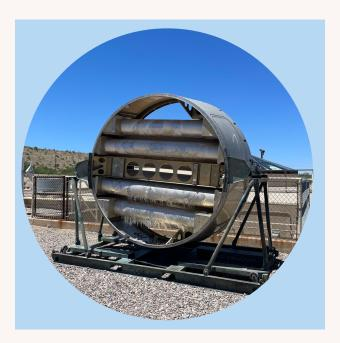
The **adapter** section paired the RV with the missile and it contained **cylinders filled with metallic balls**. These cylinders would explode upon reentry into Earth's atmosphere and above the target. The metallic balls would then be ejected around the RV in an effort to create a **decoy**, and confuse the enemy radar. The decoy mechanism was abandoned in 1975 but the cylinders remained.
