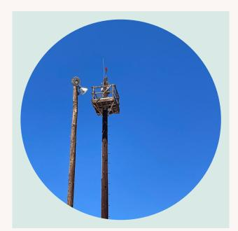
The 55-foot wooden **"Delta-T" pole** with the crows-nest on top was used together with an anemometer, which captured the speed of the wind and its direction. This was an important aspect, as weather conditions would need to be assessed before and during fueling and defueling the missiles' highly toxic propellants. The Delta-T pole was also fitted with sensors to gauge the atmospheric air pressure and temperature, as these two factors were critical in the fueling and defueling process.
